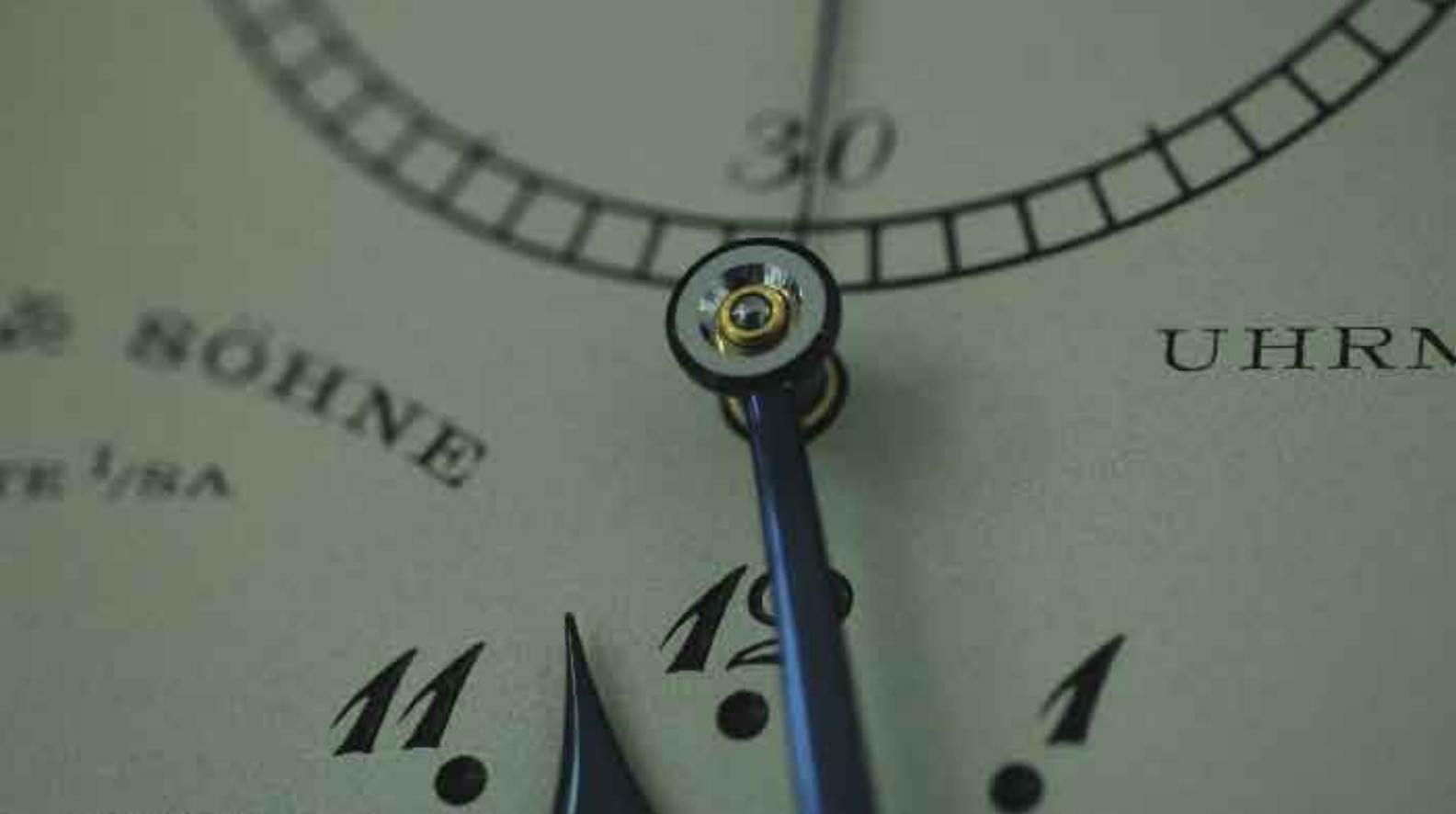
A close look at the finely blued hands made by A. Lange & Sohne in Glashutte.
